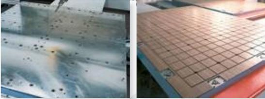
Aluminum flat surface table Phenolic resin grid table
