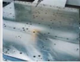
Aluminum flat surface table with grid holes or threaded inserts
