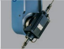
6 kW DFM milling spindle
