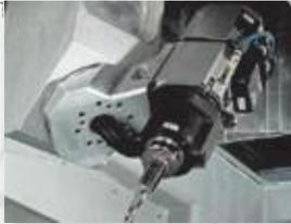
Milling spindle, HSK F63, 10 kW or 15 kW
