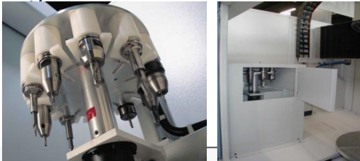
Trammel -type magazine with 10 tool places
